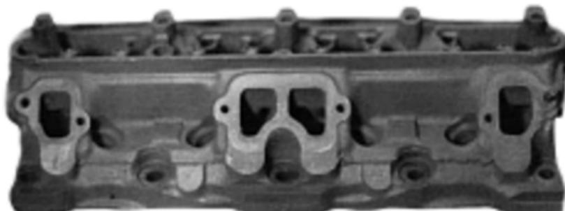
The LA-series heads are of an inline valve configuration actuated through rocker shafts. This head, number 3671587, is made for the 1973 340-cid and 1974 360-cid engines.
